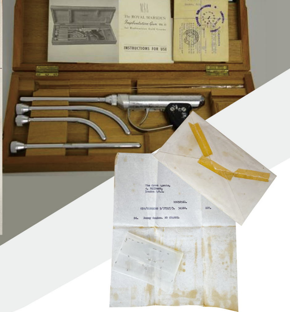
The ROYAL MARSDEN Implantation Gun Mk II for Radioactive Gold Grains A. Switch B. Needle, Nose and Spring, Straight and Curved C. Magazine with End Cap D. Lever and Plunger for long and short needles E. Rammer Applicator F. Nylon Pad G. Loading Platform H. Handle Guard
